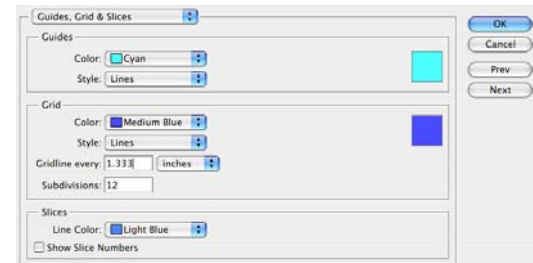
Figure 7. These grid settings will assist in aligning roll segments and keeping tracks vertical.
