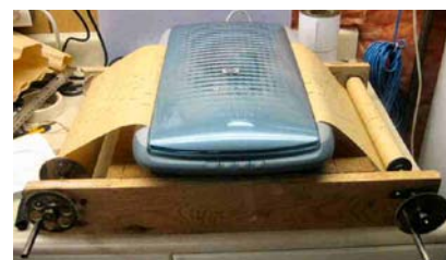
Figure 4. People already involved in piano roll repair will likely have a hand-cranked "rig" that can be easily adapted for scanning. A flatbed scanner can be mounted on its surface, and the roll repair rig's spool mechanism will make paper handling much easier.
